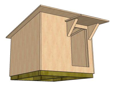
Note: The roof overhangs the front by 4" and the sides and back by 2"
