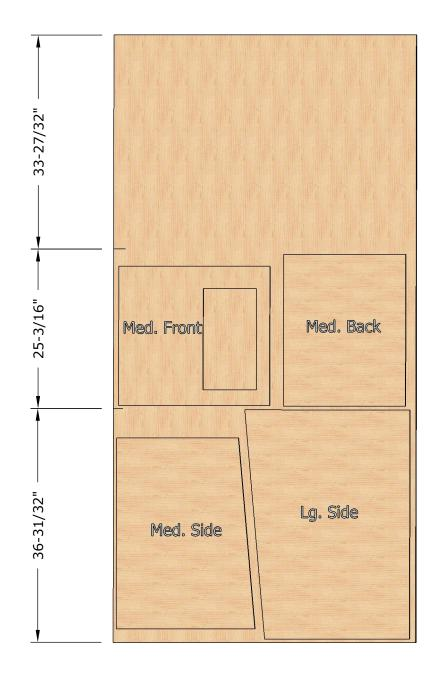
Again, this shows the components that can be cut from this sheet and the dimensions are just for potential "first" rough cuts. The left over piece may be used for mistakes or components for other houses.
