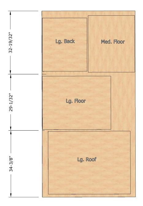
This shows the components that may be cut from this sheet of the 4'X 8' OSB. Their dimensions are provided on other pages to accommodate finish cut to size.
