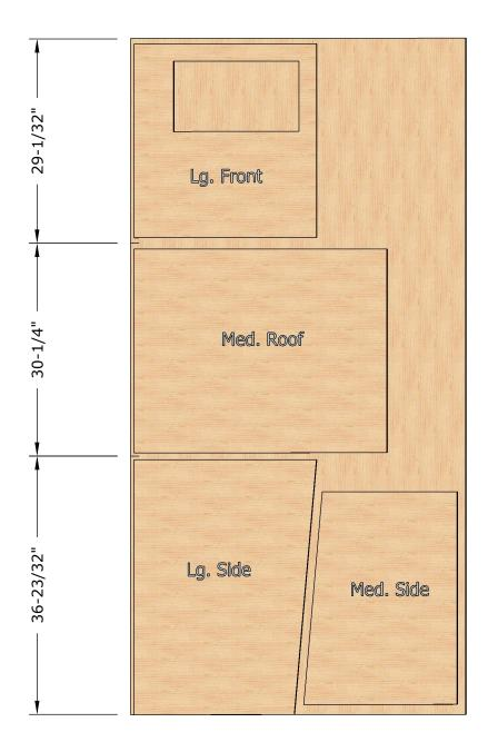
Again, this shows the components that can be cut from this sheet and the dimensions are just for potential "first" rough cuts.
